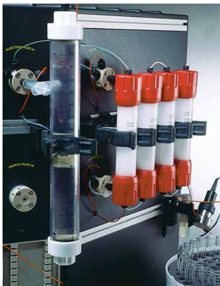
Fig 10. Four HiPrep 26/10 Desalting columns connected in series.
